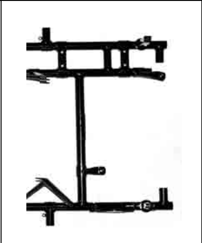
Foto from above of the frame with the section of the two supports for the RTPS (Rear Tire Protection System)
